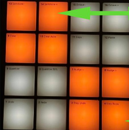
Pad turns orange when FX Unit is ON/
