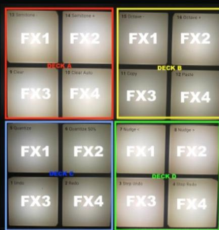
FX Units 1-4 On/Off For Decks ABCD
