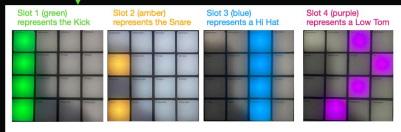
TIP: to erase a step simply press the step (pad) you want to erase. To erase all STEPS on a SLOT, press and hold [SHIFT] and the corresponding [SEQ\_] button at the top of the right screen and it will remove all steps on that slot only.
