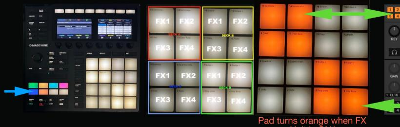
Press PAD E For FX Units FX Units 1-4 On/Off For Decks ABCD
